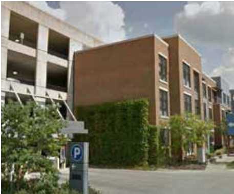
Other uses, such as the townhomes shown here, retail, or office, can be used to screen parking structures.
