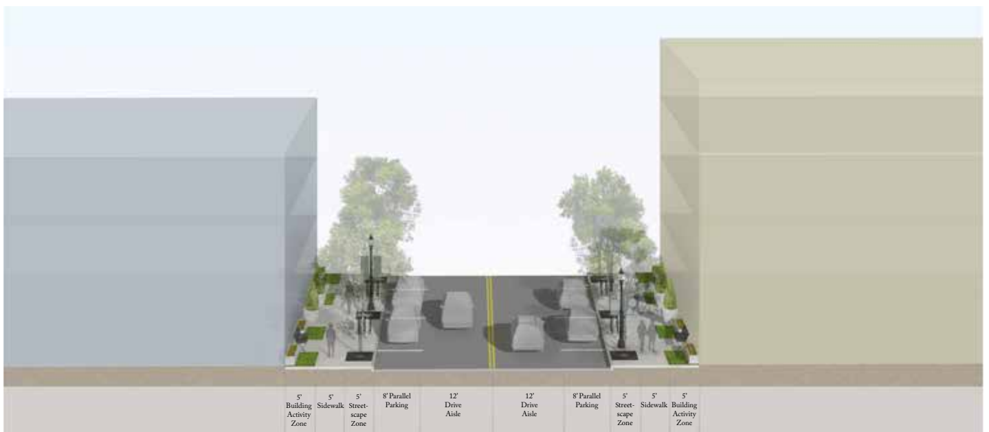
2B Secondary Roadway with Paved Streetscape Zone
