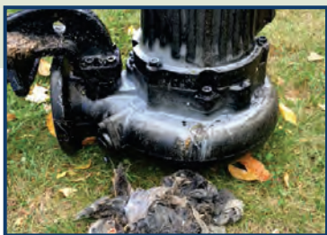
Never put "disposable wipes" down a drain or toilet - they cause costly blockages in sewers.
