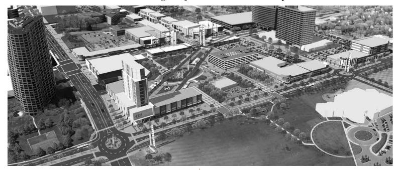
The \$12 million Evergreen Road Improvement Project is fast nearing completion. The road is expected to be fully open by September 15 with additional amenities completed by the end of October. The Project involved the total reconstruction of a one-mile segment of Evergreen Road between 10 and 11 Mile Roads from the previous six and seven-lane road into a new four-lane boulevard with a roundabout at Civic Center Drive and at the north Municipal Campus driveway.
